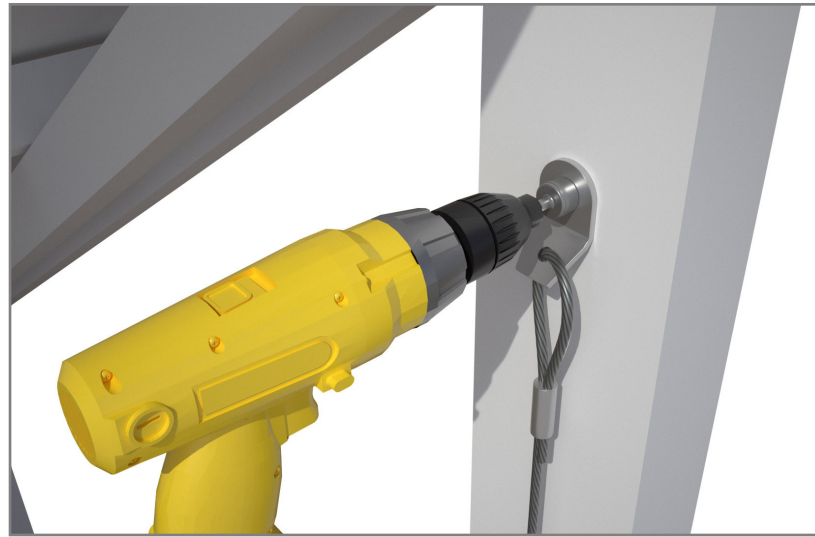
Fix eyelet end fixings to the frame.
