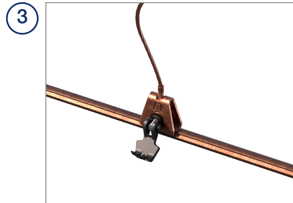
Fix the Contact Clamp to the Contact Wire by placing the Clamp onto the anvil and flipping the lever to apply clamping force. The two hooks should hook fully over the Contact Clamp (as shown).
