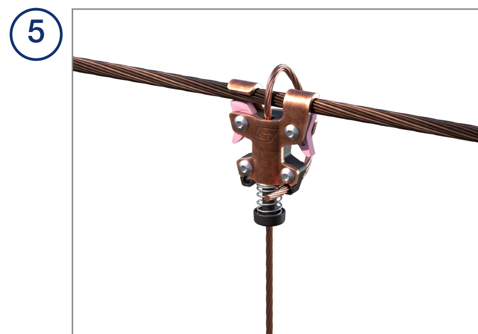
Wrap the excess wire which is above the Top Dropper around to the opposite side of the housing and push it through the lower hole (as shown) to allow it to operate as a fail safe.
