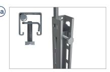
Rotate and engage into Universal Bracket or Strut return
