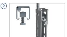
Insert rod stiffener clip into Universal Bracket or Strut as shown
