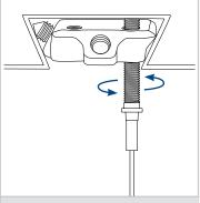
4) Insert Stud hanger into the wedge, ensuring it is tightened into the decking
