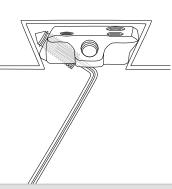
Tighten the screw into the decking profile, using an allen key
