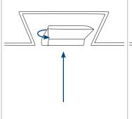
2) Insert wedge nut into decking channel and rotate 90°
