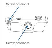
Manually insert the screw into the desired position (see table)
